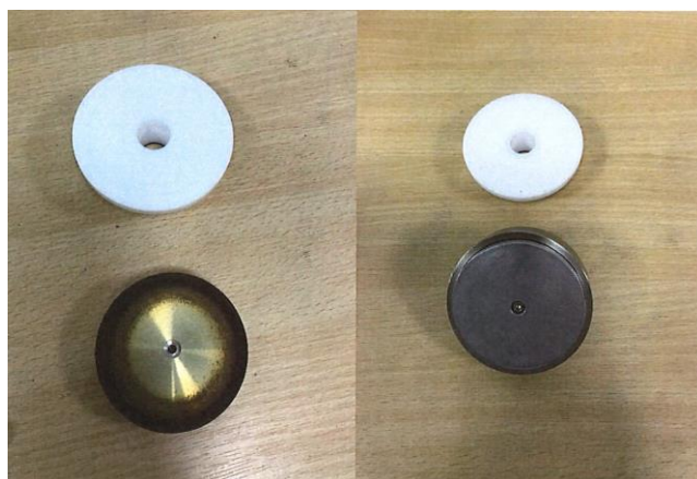
Figure 7-6. Glow discharge head: (left) before cleaning and (right) after cleaning
