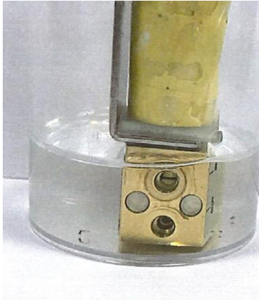
Figure 7-3. Cleaning a vapour valve in isopropanol
