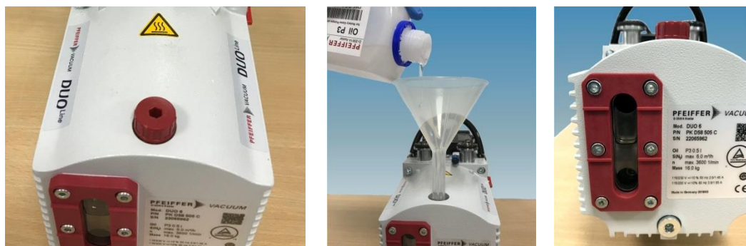
Figure 2-2. Filling the rotary pump with oil (left) Red screw cap on top of rotary pump (centre) Filling the pump with oil (right) Oil level gauge on side of pump
