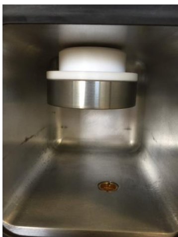
Figure 7-5. Glow discharge head: (left) in position and (right) removed
